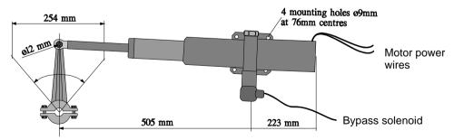
**Warning!** A strong mounting bracket must be made for the Linear Drive trunnion mount since forces up to 600 kg (1400 lb) can be developed.
