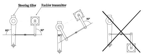
Small errors will not affect Autopilot operation but will cause inaccurate indication on the rudder angle indicator. If possible, the linkage on the rudder transmitter should be adjusted so that the digital rudder angle indicator on the Instrument display is consistent with the rudder angle. The cable should be connected to Servo Unit terminals marked "RFU" according to colours indicated.
